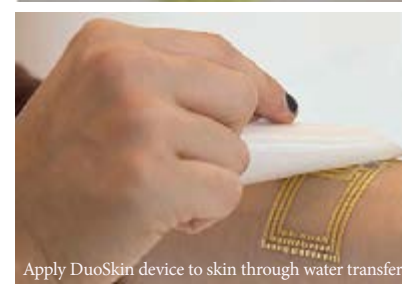
Apply DuoSkin device to skin through water transfer
